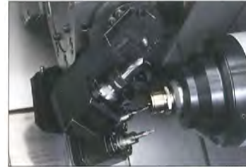
Skewed Hole Drilling
