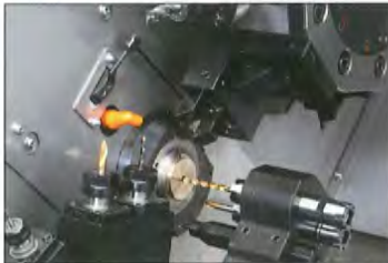
Machining and Positioning of the Twin Turrets
