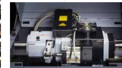
Built-in motor[for main spindle]
