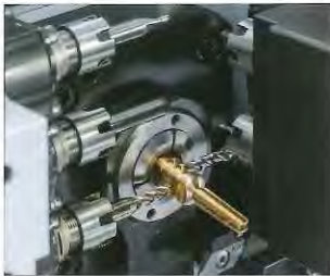
Reduced cutting time by simultaneous machining
