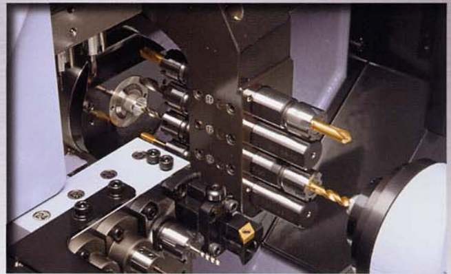
Main/sub spindle simultaneous drilling
